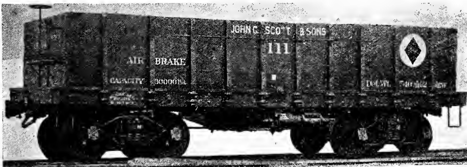
Fig. 25. GONDOLA CAR, WITH PYRAMIDAL HOPPER-BOTTOM, FOR COAL. Length, 26 ft. Capacity, 60,000 lbs. Weight, 23,400 lbs. Equipped with Air Brake, Side Trussing and Rigid Diamond Trucks.
